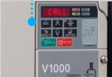
Stirrer rotation inverter working at 9 different speed levels, from 7 up to 70 Hertz. Many different products, even the most delicate, are now possible thanks to PLC and inverter as well as a perfect batch freezing depending on the produced quantities and features of the mix and on the ingredients and their mix formulation.
