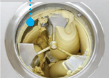
The stirrer rotation direction does not change according to speed. Therefore the machine mechanical operation is much more reliable over time.
