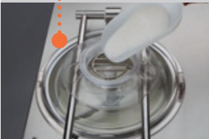
Double lid with opening system actuated by servo-assisted hydraulic pistons for easy ingredient introduction even in case of product in progress. The machine has not to be stopped in full compliance with certified EC safety regulations.
